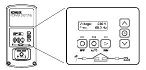
The RDC2 controller provides integrated control for the generator set, Kohler® Model RXT transfer switch, programmable interface module (PIM), and load control module (LCM).
